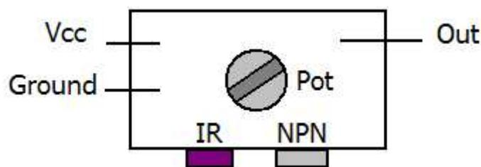
*Fig. 3: Line detection Module*
